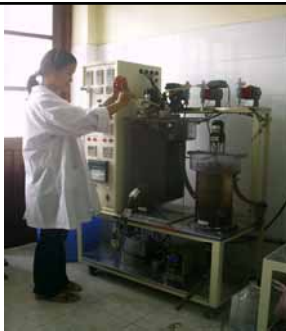
Treatment of beery wastewater by activated sludge process
