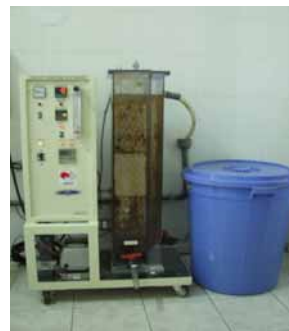
Removal of organic pollutants from textile wastewater by contact oxidation process
