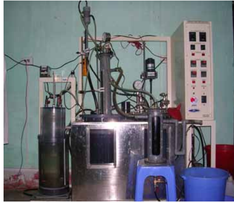
Treatment of beery wastewater by UASB process
